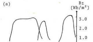
Fig. 4. Magnetic field distribution along the axis. (a): main compression field. (b): bias and guide field.
