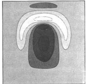
Figure 4 Contours of constant B_z across the minor cross-section at t=27 . (The contours are equally spaced between 0.70 and 1.20 of the initial constant value)
