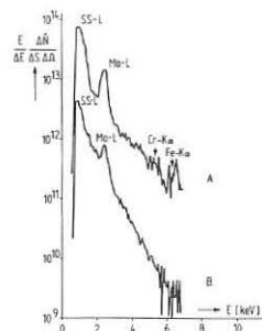
Fig. 3 X-ray spectra of discharges A and B integrated between 60 and 120 ms
