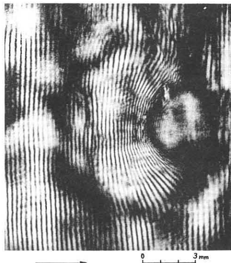
Fig. 1. Holographic interferogram of the laser-produced solid target plasma in vacuum at t = 100 \text{ ns} .
