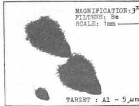
Fig. 3. Pin-hole image of thin foil plasma in 3 frames.
